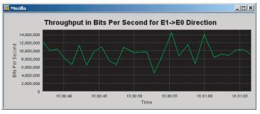
Users can also easily display real-time throughput in bits/sec. and packets/sec. on each port in both tabular or graphical format. Throughput numbers are very accurate as they are collected from the Network Emulator's kernel application. In other words, while the emulation is heavily taking place the throughput numbers would still be very reliable.
